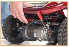
To separate the rear transaxle from the frame, squeeze the release lever located on the underside of the frame
